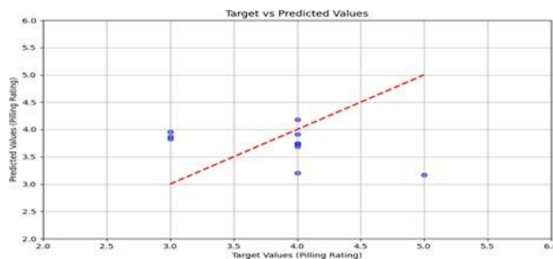
Figure 11. Correlation between actual and predicted value of pilling rating using root mean square error function.
