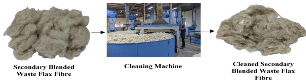
Figure 3. Cleaning of the secondary waste flax fibre using a waste-treating machine.
