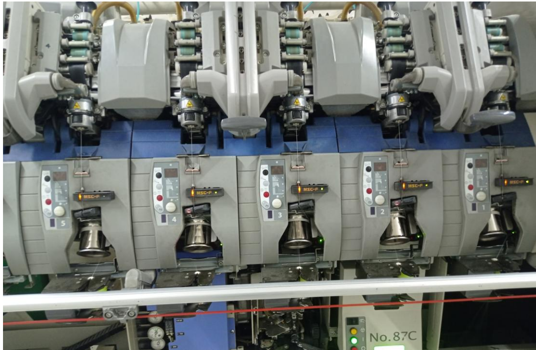
Figure 2: Yarn formation zone of vortex spinning (MVS)
